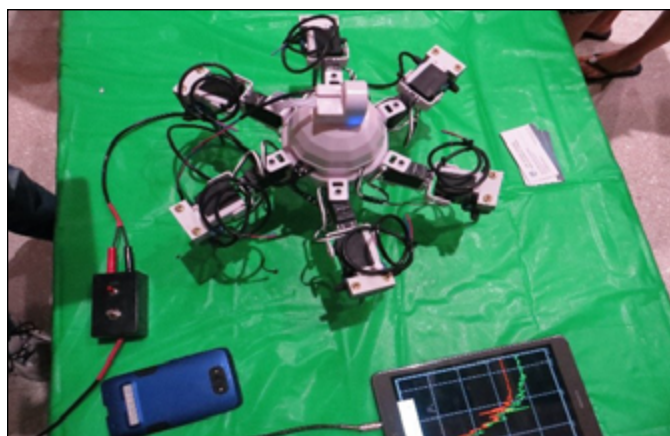
Robot geophone used to demonstrate recording of seismic waves
